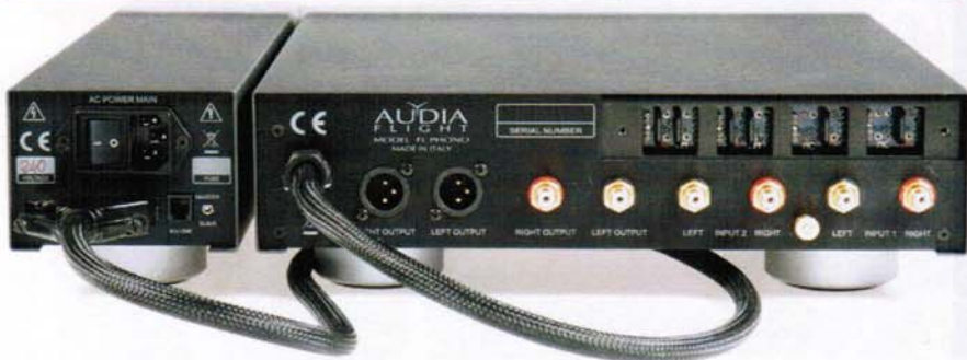
ABOVE: Both single-ended (RCA) and balanced (XLR) outputs are provided, while the two inputs can be selected via a push button on the fascia. RJ45 socket on the power supply provides a comms link with Audia's amplifiers for automatic power on/off
