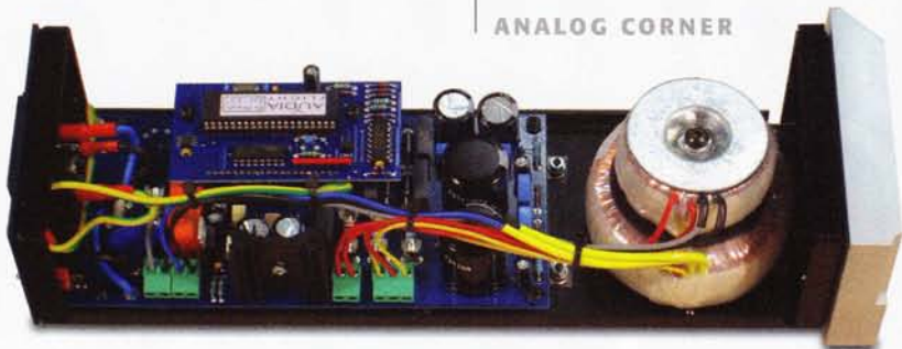
Inside the Audia Flight's power supply.
